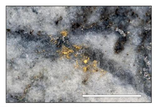
ES17-64: Native gold with arsenopyrite. Core sample at - 204.65 m downhole.
