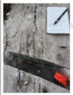
Tonalite with generally less than 1% arsenopyrite and pyrrhotite as disseminations or veinlets. Strongly silicified tonalite carrying 3 mm to 10 mm wide clusters of visible gold, partially controlled by a tight quartz-chlorite stockwork and moderate biotite alteration
